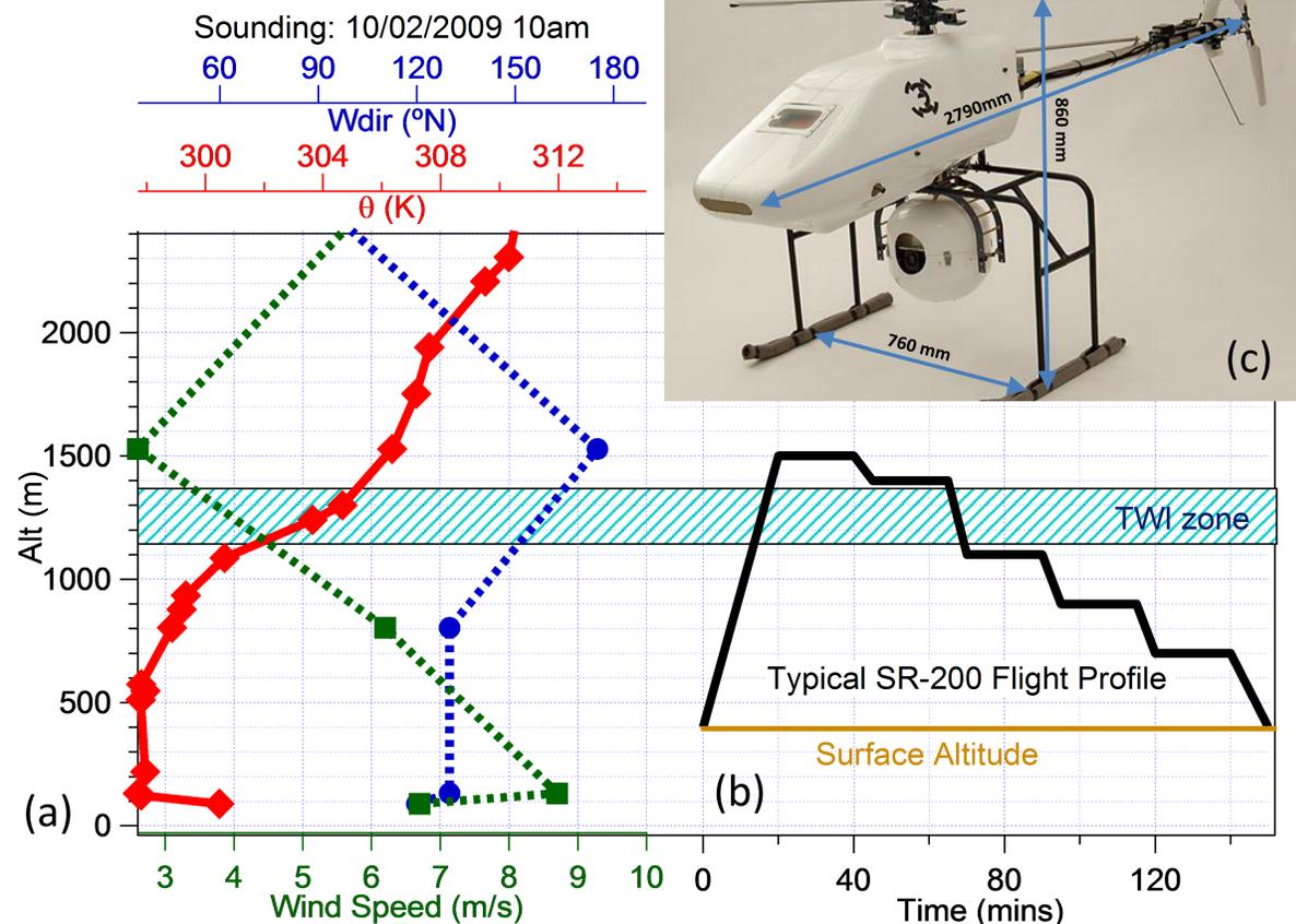
Figure 2: Potential Temperature ( $\theta$ ), Wind Speed and direction balloon sounding from February 2009 compared with typical planned flight profile for Ascension Island RPV campaign. SR-200 RPV system is shown in (c).
