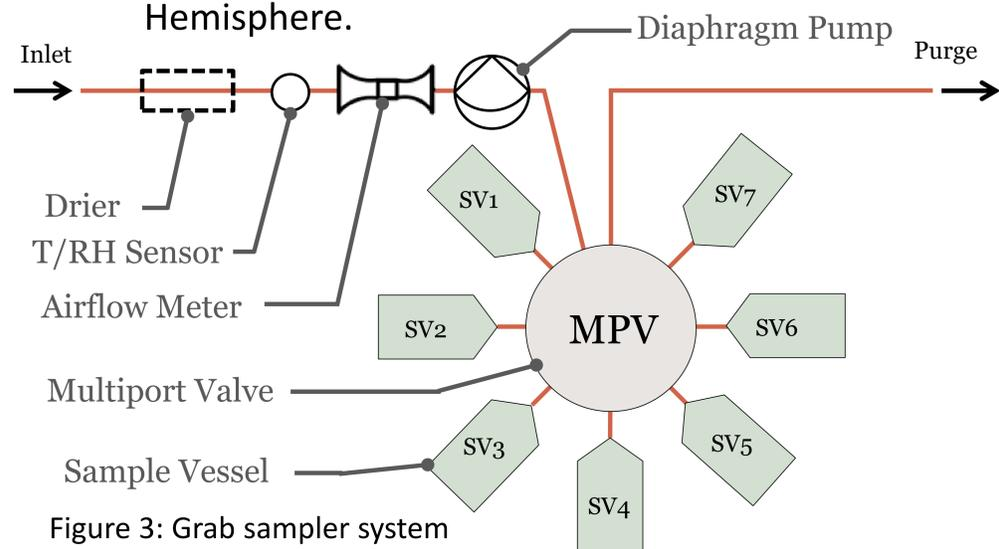
Figure 3: Grab sampler system air flow schematic
