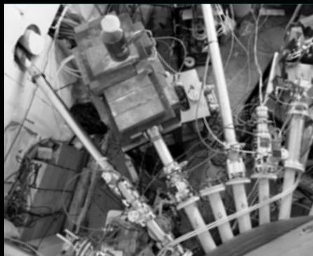
In practice, the maximum achievable proton energy is around 38 MeV. Helium-3 is run using the recirculating gas system acquired from the decommissioned Hammersmith cyclotron; the MC40 vacuum is maintained using a single diffusion pump whose exhaust is passed through a cold zeolite filter and then returned to the ion source. Additionally, small beams of 46 MeV  $^{14}\text{N}^{4+}$  and 71 MeV  $^{14}\text{N}^{5+}$  have also been extracted and used for nuclear physics studies.
